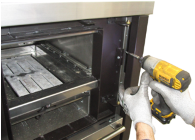
Fig. 28 - Retirer le support
